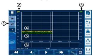
1 Selection keys for showing one or two measured variables Pressing a key activates or deactivates display of the respective measured variable.
