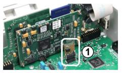
The configuration module is plugged in to a plug socket, making it easy to replace or to plug into another unit.
