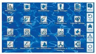
Every function is represented by an icon with supplemental text (The set of icons shown depend on the controller model).
