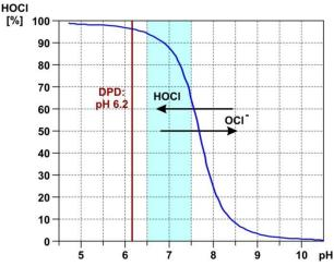
If control measurements are performed using the DPD method, then it is important to know that the DPD measurement is always performed at a pH value of ca. 6.2. That value is attained with an integrated pH buffer in the DPD reagents. Thus, a DPD measurement always measures all free chlorine independently of the actual pH value in the pool. Therefore, a DPD measurement may not be significant for the real disinfection effectiveness, especially, if pH is above ca. 7.5.
