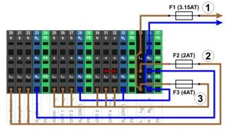
The supply for the Analyt unit as well as for the alarm relay and the add-on functions share a mutual power input (L/N). Phase L for Analyt is run from the input over via fuse F1. Phase L<sub>F</sub> for the alarm relay and the add-on functions is run from the input via fuse F3. Neutral conductors N and NF are connected to each other internally.
