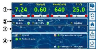
1 Measured value display with additional graphic measured value scale
